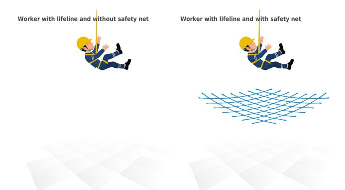
In comparision to individual protective system, the worker is always safe, while using other individual systems such as lifelines, temporary or definitive, the worker is safe just when he is attached.
